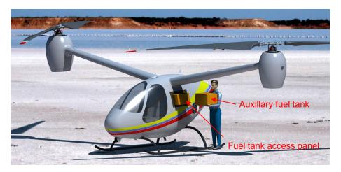
FIGURE 11.10: Main and auxiliary fuel tank placement.
